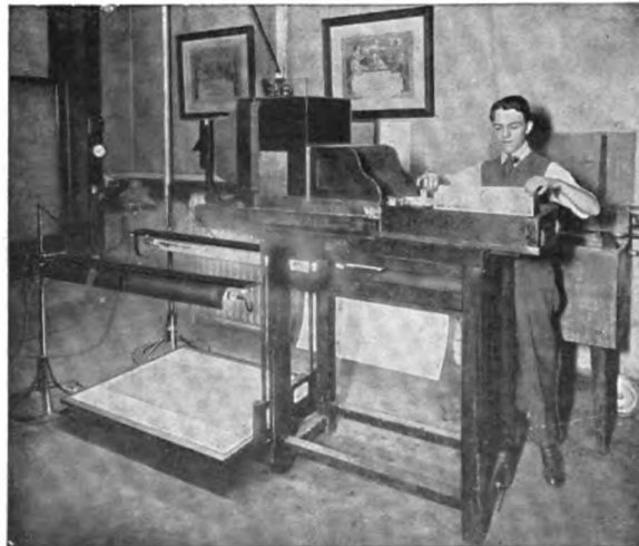
This Cut Shows a Photostat Installation
